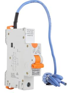
NHP MOD6 Residual Current Device - Short body w/ Overcurrent 6kA 16A 1PN C Curve 30mA Type A Pigtail
