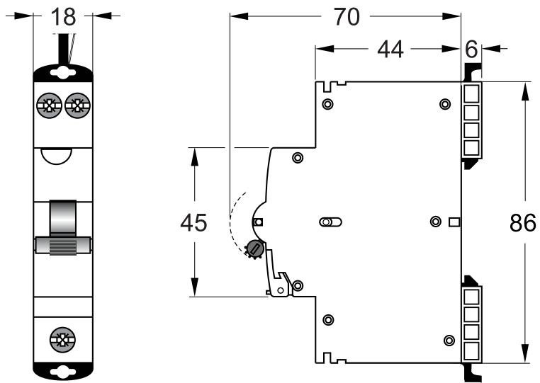
NHP MOD6 Residual Current Device - Short body w/ Overcurrent 6kA 16A 1PN C Curve 30mA Type A Pigtail
