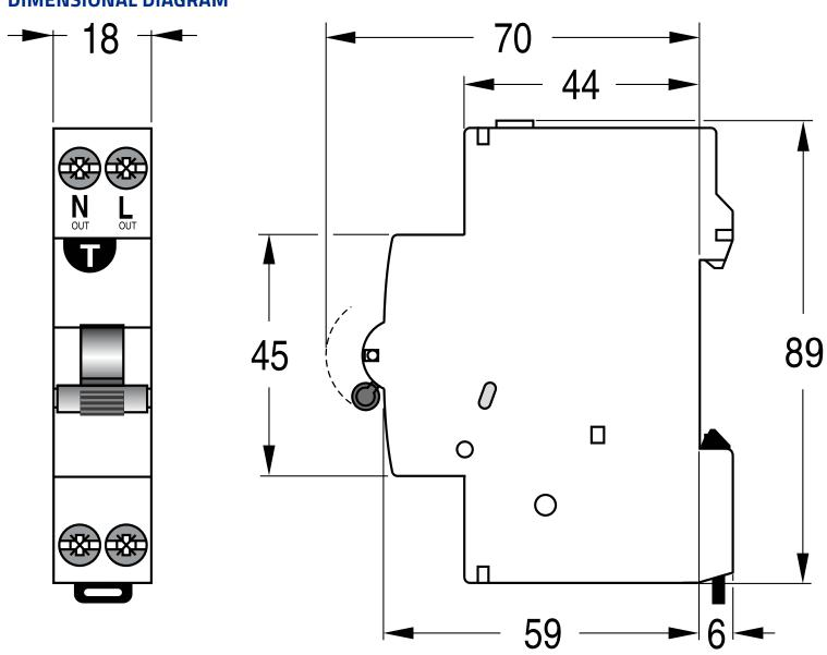
NHP MOD6 Residual Current Device - Short body w/ Overcurrent 6kA 10A 1PN C Curve 30mA Type A 2 Screw
