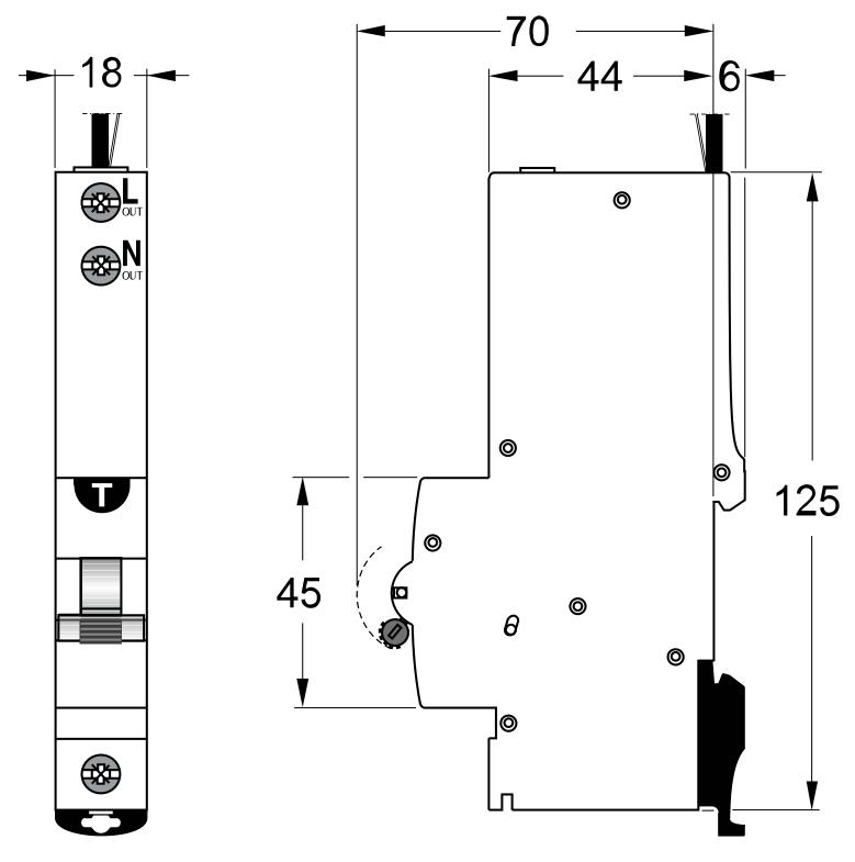
NHP MOD6 Residual Current Device - Long body w/ Overcurrent 6kA 32A 1Pole and N C Curve 30mA Type A
