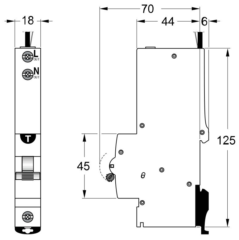
NHP MOD6 Residual Current Device - Long body w/ Overcurrent 6kA 25A 1Pole and N C Curve 30mA Type A
