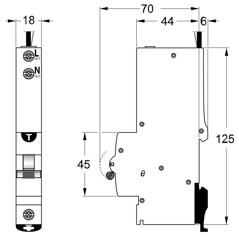
NHP MOD6 Residual Current Device - Long body w/ Overcurrent 6kA 16A 1Pole and N C Curve 30mA Type A
