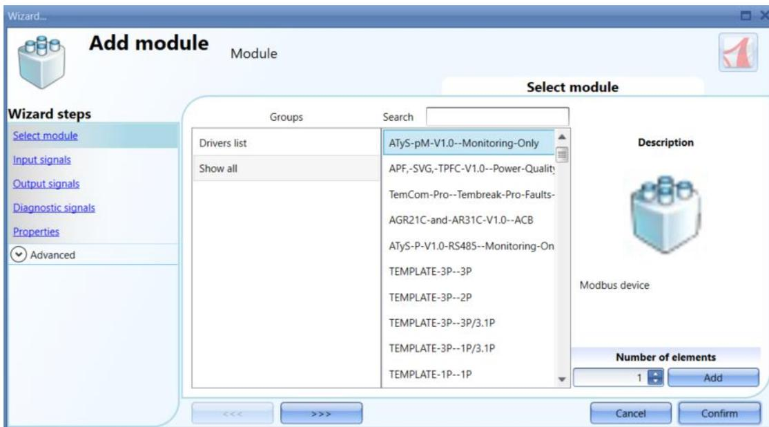
8. Before clicking on confirm go to properties and check the Modbus ID matches that of the ATyS p M module (please refer to Section 13.9 on page 65 of the ATyS p M instruction manual for communication address and designation details.) Click confirm.
