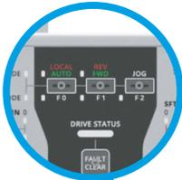
HOA keypad for local control when PLC is not available. Buttons are user-programmable for more flexible local control.
