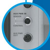
Feed-through 24V DC auxiliary power supply lets you configure the device even when 3-phase power is off. Optional internal power supply.
